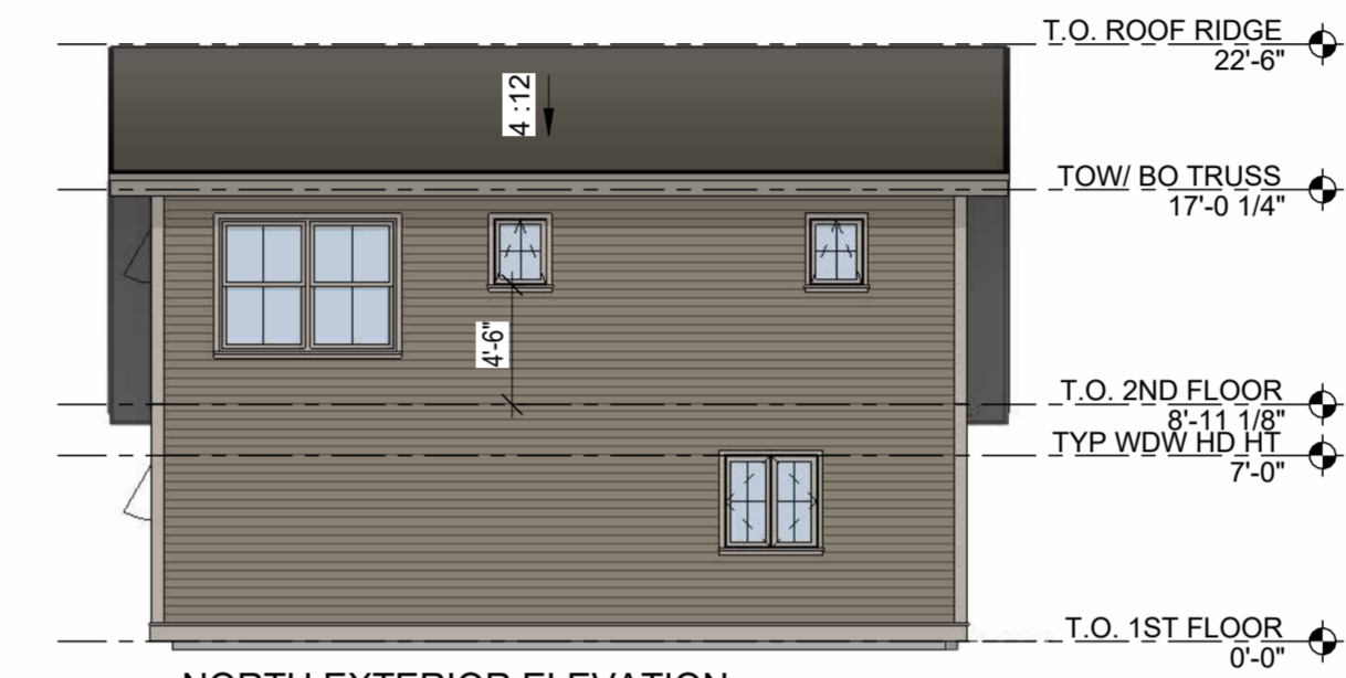
⑤ NORTH EXTERIOR ELEVATION 1/8" = 1'-0"
